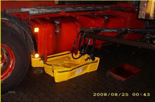
Diesel oil leaking from truck tank
